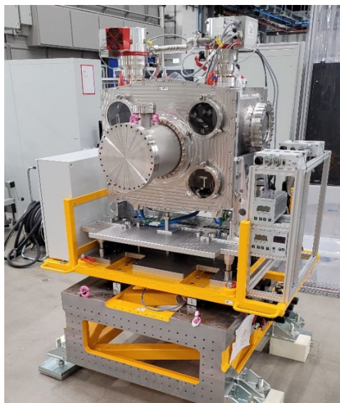
Figure 1: Assembled MDS on separate girder. Including the vacuum chamber with the detectors inside and the tray for electronics
