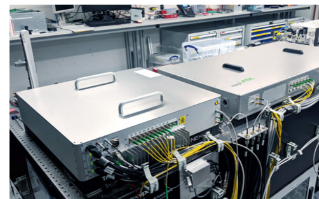
Figure 1: Fibre frontend and power amplifier of the NEPAL-X1 laser during installation
