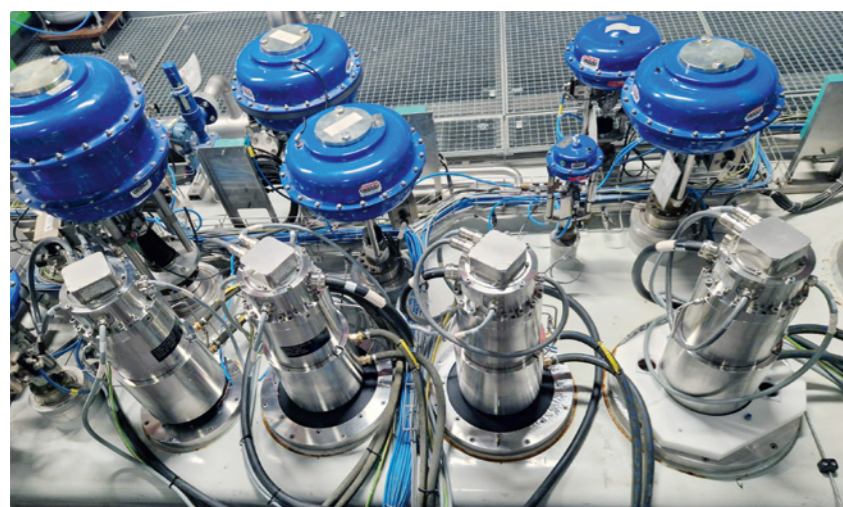
Figure 1: Cold compressor motors with active magnetic bearings (metallic pillars in the front) installed in the 2 K cold box
