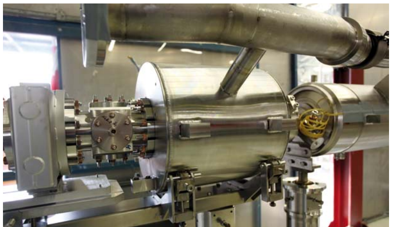
Figure 7 Cold magnet prototype for the Cold Magnets WP of the Linac WPG
