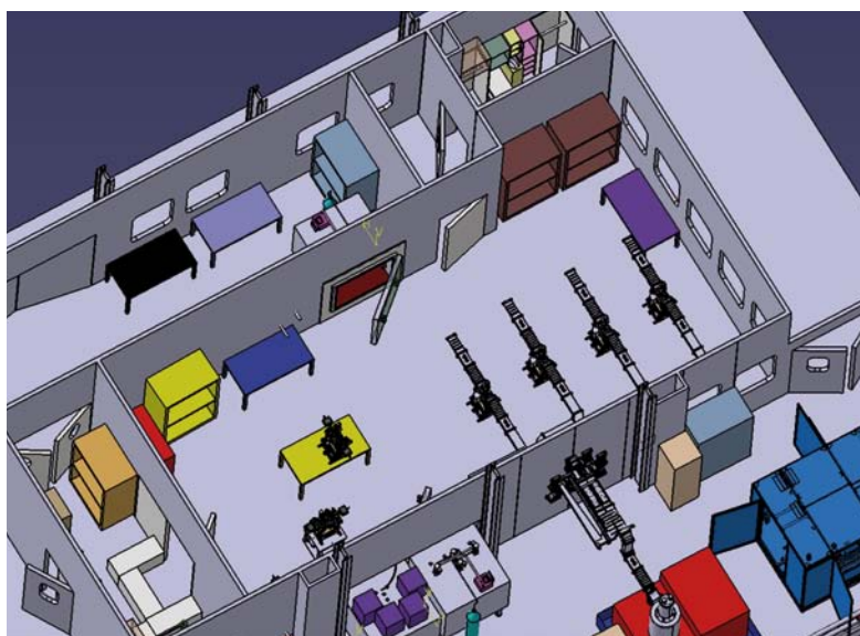
Figure 2 New CNRS-LAL Orsay infrastructure to be used for the RF power coupler conditioning
