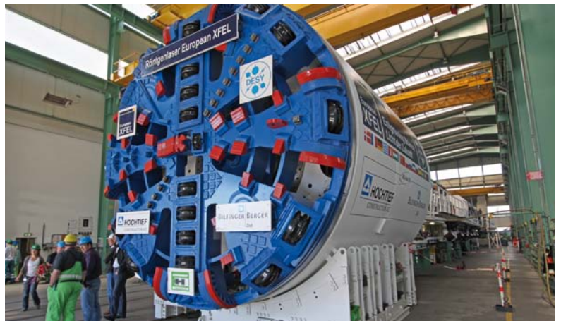
Figure 8 Smaller tunnel boring machine, AMELI, after its test assembly at the manufacturer
