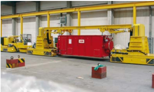
Figure 6 Transport vehicle for the pulse transformer
