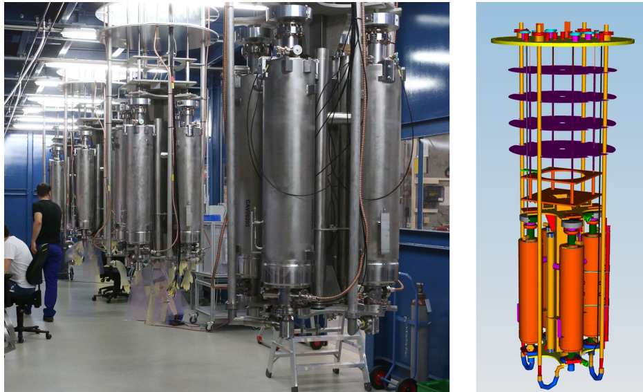
FIG. 5. Left: vertical test inserts ready for test. Right: 3D view drawing of a test insert supporting four equipped cavities.
