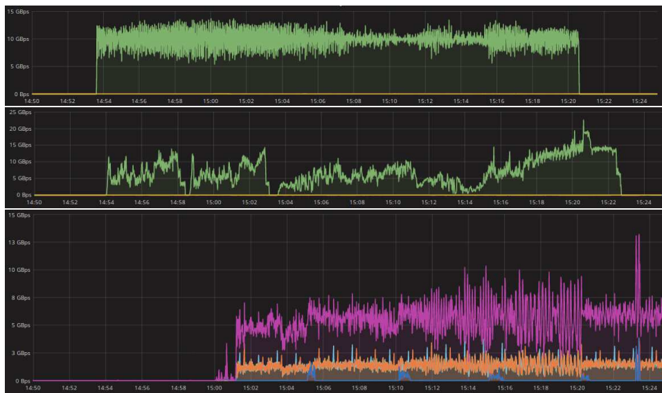
Figure 3. Throughput (GB/s) in function of time of three processes: the top picture – the simulated data ingest from PC-Layer cluster integrated over all nodes; the middle picture – simulated data ingest from on-line analysis cluster integrated over all nodes; the bottom picture - the data copy process (read) from on-line to off-line cluster, the magenta line denotes integrated throughput, other colors each node individually.
