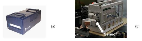
**Figure 3**. Two LPD detector prototypes are shown. (a) LPD 2-Tile detector prototype with  $32 \times 256$  pixels, and (b) LPD supermodule detector prototype partly populated with sensor tiles resulting in a  $256 \times 256$  pixels geometry.
