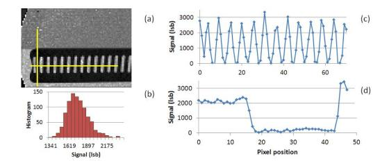
**Figure 4**. Large area signal exposure on two tiles of the detector. (a) Cu fluorescence image of a Jubilee clip. Yellow lines indicate where the profile plots are taken. (b) Histogram of a uniform ROI in the upper part of the image. (c) Horizontal profile of clip. (d) Vertical profile of clip.
