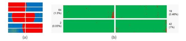
**Figure 5**. Pixel map of non-responsive pixels. (a) Scan of beam (in red) across tiles in three steps. (b) Defective pixels are shown in red. The number of defects per tile and its percentage value are given.
