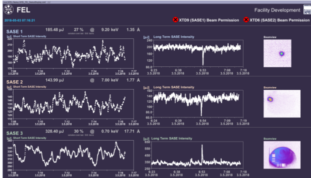
Figure 1: Screenshot of the SASE level display of European XFEL with all 3 SASE lines in operation. On the right hand side images of screens in photon beamlines can be seen.
