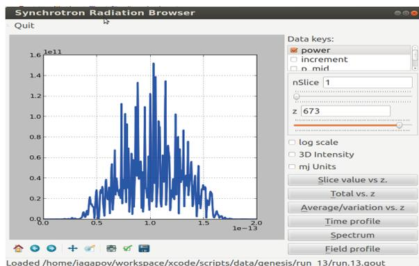
Figure 2: Xframework contains a graphical (Qt4-based) postprocessing tool supporting plotting basic simulation output. More complicated operations are accessible from python scripts.
