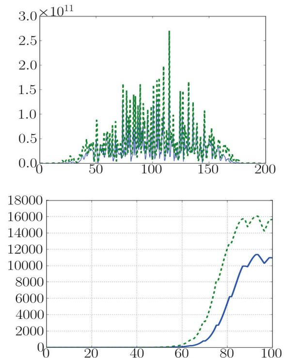
Figure 1: Output signals corresponding to 4KA (solid line) and 5KA (dashed line) input current, for the same seed, SASE3 undulator.
