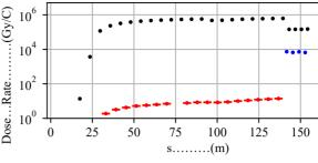
Figure 1: Dose rates in the copper absorbers (black), the planar undulators (red) and the Apple-X undulators (blue).
