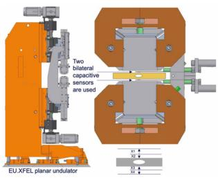
Figure 1: Layout the planar undulator (left) and the gap measurement unit (right).
