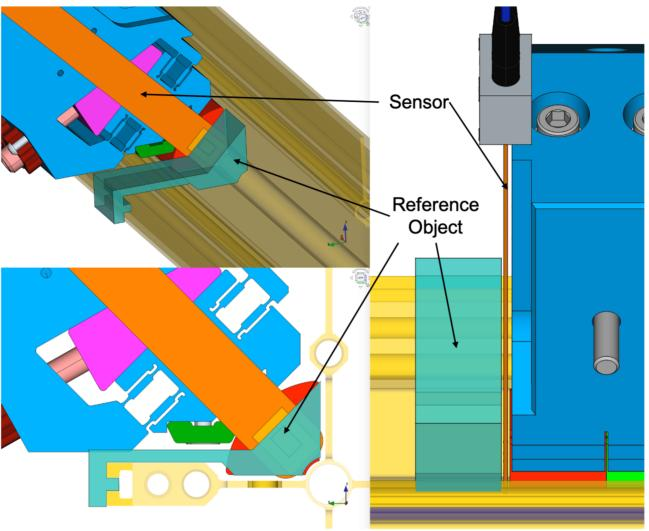
Figure 4: Isometric (top left) frontal (bottom left) and top (left) views of the shift measurement setup.
