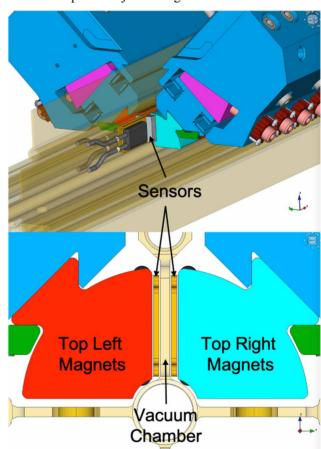
Figure 3: Isometric (top) and frontal (bottom) views of the gap measurement setup.
