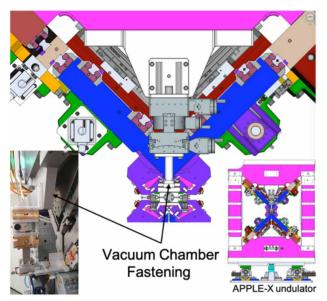
Figure 2: Layout of the vacuum chamber fixation for the APPLE-X undulator.
