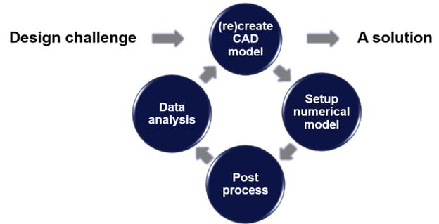
Figure 4: Conventional design workflow.
