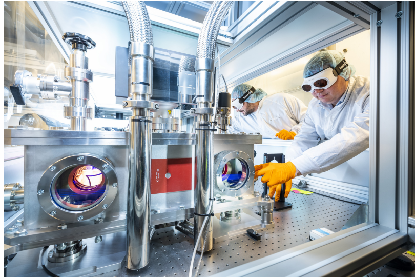
Figure 1.12: HZDR HIBEF scientists Toncian and Höppner aligning the last amplifier of the ReLaX laser system
