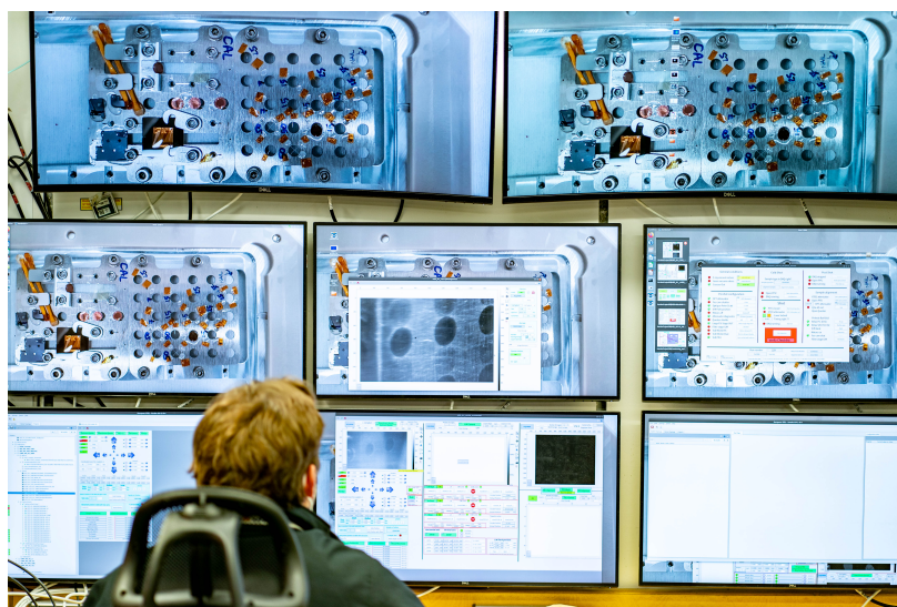
Figure 1.26: HZDR HIBEF instrument scientist A. Pelka operating the HED-HIBEF instrument in the instrument control room. The top screens show the solid targets arrangement. The screen in the centre shows the live view of the targets in IC1.
