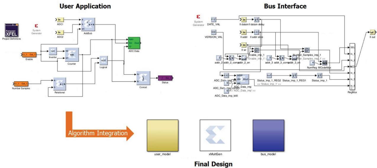
Figure 4: Design example. The Bus Interface logic is generated during Algorithm Integration based on user defined registers. The bus\_model block includes the Bus Interface logic while a copy of the original algorithm is wrapped on the user\_model block.
