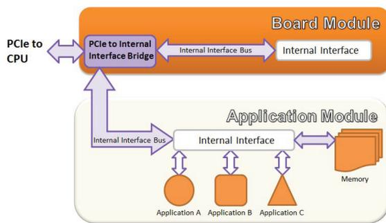
Figure 1: FPGA projects structure.
