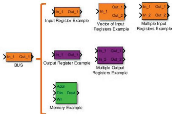
Figure 3: BUS block example. The block regenerates according to the parameters defined by the user.
