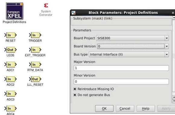
Figure 2: Board definition in a Simulink project.
