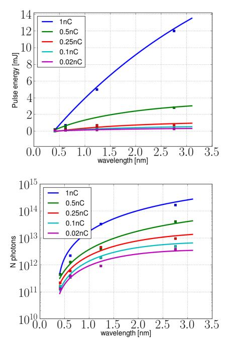
Fig. 1. SASE3 baseline for 14 GeV electron energy: (top) pulse energy and (bottom) number of photons per pulse as a function of photon energy and bunch charge in the SASE saturation mode of operation.
