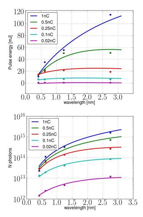
Fig. 2. SASE3 baseline for 14 GeV electron energy: (top) pulse energy and (bottom) number of photons per pulse as a function of photon energy and bunch charge in the SASE tapering mode of operation.
