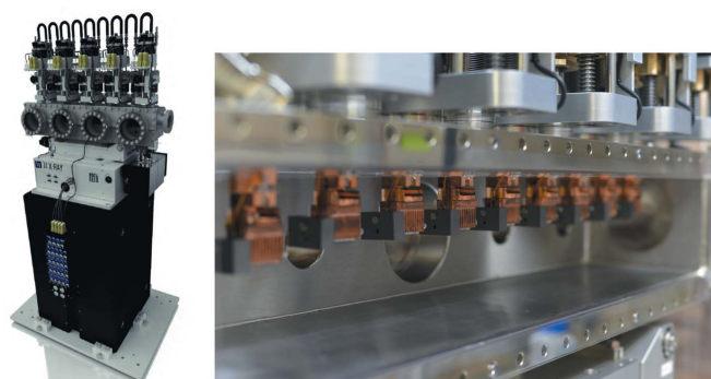
Figure 3 CAD-model of the JJ X-ray translocator unit (left) and photograph of the lens cassettes inside the chamber installed in the XTD9 tunnel (right).
