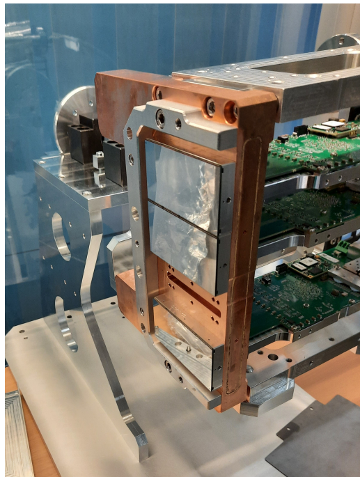
Figure 3.7: The Jungfrau 4Mpix during replacement of a front-end-module. The specialized stand allows easier access to all the components.
