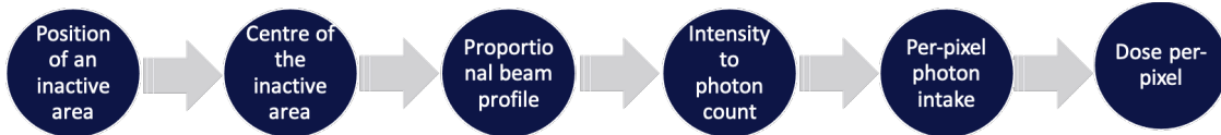
Figure 9.5: Flowchart of the analysis steps to calculate the per-pixel intake of the incoming photons throughout the course of the irradiation experiment.
