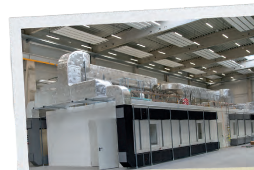
Figure 1: Measurement hutches inside the new undulator hall. In them, the magnetic measurement of the undulator segments will be performed under well-defined thermal, vibrational, and magnetic field conditions.
