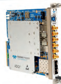
Figure 5: MicroTCA card for high-speed digitizers
