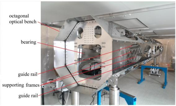
Figure 2: The SDU during the construction phase.
