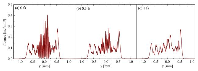
Figure 6: A vertical cut through the interference pattern for three different delays at (a)  $\Delta t = 0$  fs, (b)  $\Delta t = 0.21$  fs, (c)  $\Delta t = 1$  fs.
