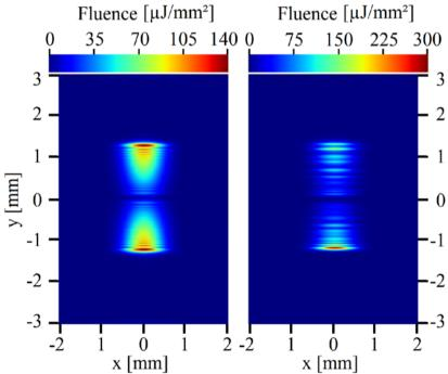
Figure 5: The two partial beams on the detector for a photon energy of hv = 15 keV with perfect mirrors in the SDU (a) and for mirrors with the mirror profile (b).
