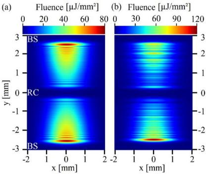
Figure 4: The two partial beams on the detector for a photon energy of hv = 5 keV with perfect mirrors in the SDU (a) and for mirrors with the mirror profile (b).
