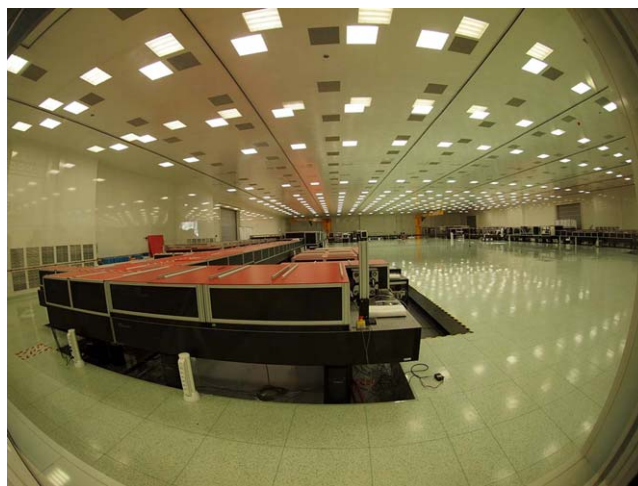
Figure 32. High power laser system (HPLS) of 10 PW 2 arms. The central laser wavelength is 820 nm with the laser bandwidth of 10 nm. The pulse width is <25 fs with 250 J laser energy output. The focused laser intensity may reach 10^{23} W cm -2 . The final laser beam size is 50 \times 50 cm 2 . HPLS sits on the vibration-dumped floor in the 70 \times 40 m 2 clean room. 100 TW or 1 PW laser outputs can be extracted for separate experiments simultaneously with 10 PW output.
