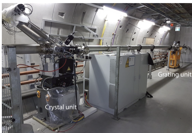
FIG. 5. Photograph of the HIREX spectrometer in the tunnel XTD9 with a safety fence around the crystal unit to protect the beryllium window against damage and to protect workers against the detector arm motion. The FEL beam direction in the image is from right to left. Upstream of the crystal unit is a dedicated electronics rack for motor and vacuum controllers.
