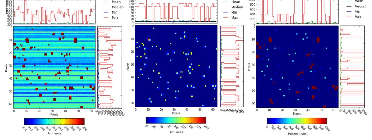
Figure 2: Examples of GPU-based corrections on test data. The left plot shows the uncorrected data with common mode effects highlighted; the center plot the same data after offset-, common mode- and gain correction have been performed on a per pixel, permemory cell basis. The right plot shows the identified patterns (classified as singles (pattern index 100), doubles (200), triples (300) and quadruples (400)), as well as clusters (1000) with higher multiplicities.
