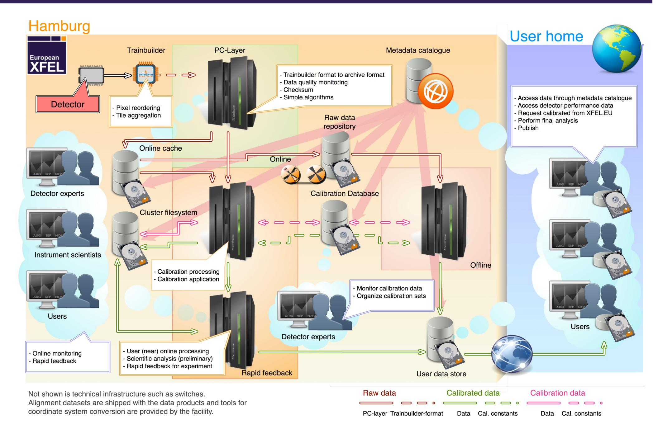
Figure 1: A general overview of data products, their flows, storage and related user roles at European XFEL, starting from data acquisition with a detector (top left corner). The different data products and formats are color-coded. Note how it is generally foreseen to provide users with calibrated data.
