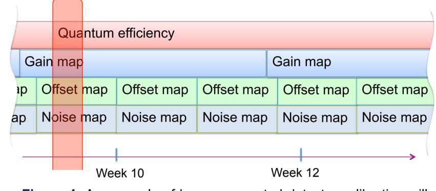
Figure 4: An example of how a requested detector calibration will map to different versions of different calibration constants.
