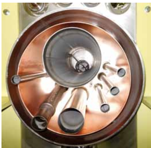
Figure 1 Injector feed cap. Cryogenic transfer line connects with the Joule–Thomson box (IKC RU24 by BINP).
