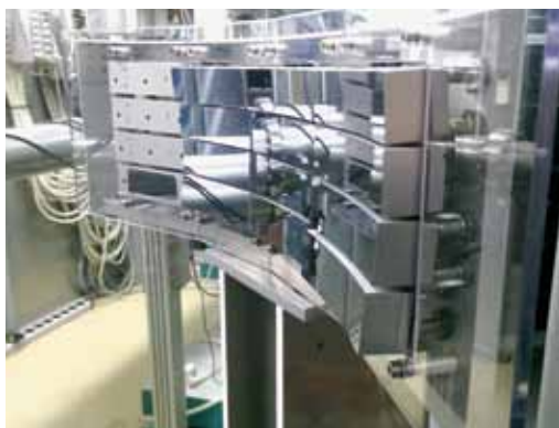
Figure 2 Von Hamos spectrometer during mounting of cylindrically bent X-ray crystals
