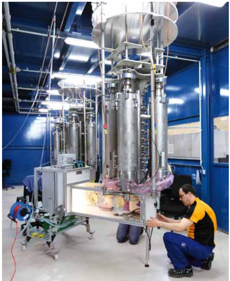
Figure 7 Setup for cavity characterization in the vertical acceptance test by a Polish team in the AMTF hall on the DESY campus (IKC PL05 by National Centre for Nuclear Research (NCBJ) in Otwock-Świerk, Poland).
