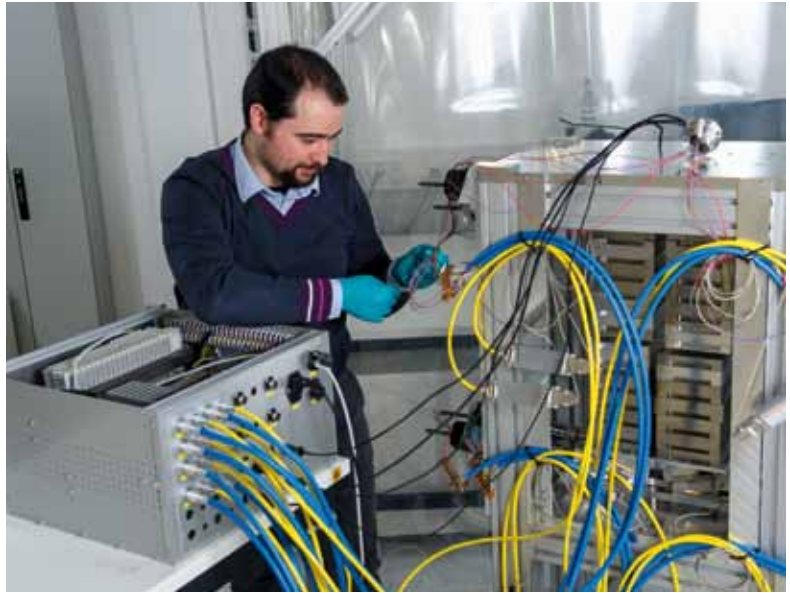
Figure 1 Test frame for the AGIPD 1 Mpx 2D detector. The four movable quadrants are visible as metallic placeholders in the centre right of the picture.
