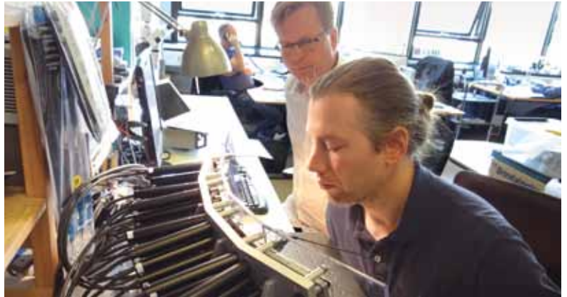
Figure 4 Tests carried out for the von Hamos spectrometer at the premises of JJ X-Ray in Lyngby, Denmark. The resolution ( 0.2 \mu\text{m} ) and repeatability ( 1 \mu\text{m} ) of motor movements were better than the specifications. The system was designed and produced by the industrial partner JJ X-Ray (IKC DK01 by DTU) for the Femtosecond X-Ray Experiments (FXE) instrument.
