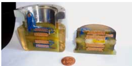
Figure 1 Cross-section of compact coils for millisecond-long magnetic pulses developed by Peter van der Linden at ESRF. The Sample Environment group will test similar electromagnets to destruction to prove their suitability for the scientific instruments.
