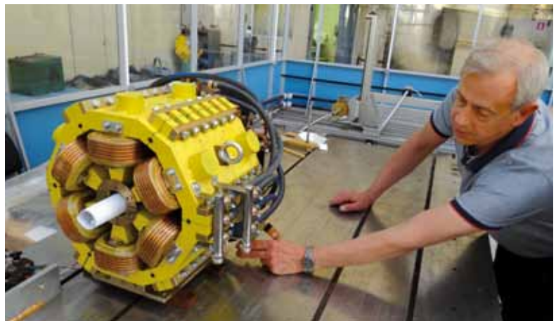
Figure 2 Sextupole magnets. The control of chromatic effects is one of the main issues in the design of the optics in the collimation section. Therefore, introduction of chromaticity-correcting sextupoles becomes essential to improve overall system performance (IKC RU11/WP12 by NII-EFA).
