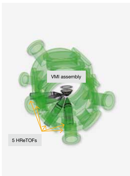
Figure 1 Sketch of the AQS experiment chamber showing the first interaction area, which is surrounded by one VMI and five HReTOF spectrometers
