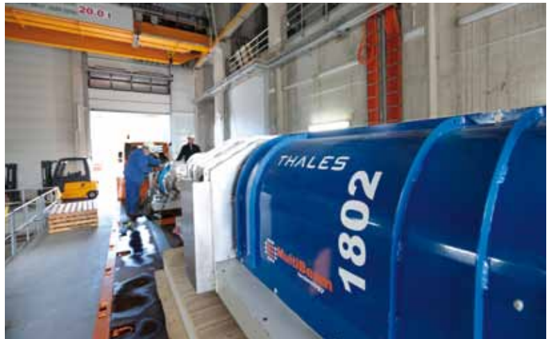
Figure 6 Klystrons stored for tunnel installation after passing the acceptance test (IKC DE01 by DESY)
