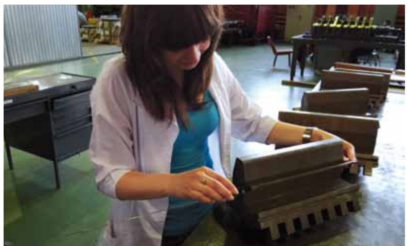
Figure 3 Production of XQF quadrupole magnets in St Petersburg, Russia. The quadrant is measured before assembly with a precision of 0.5 mm (IKC RU11/WP12 by NII-EFA).
