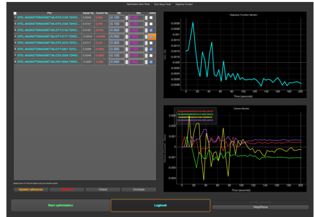
Figure 6: SASE tuning with 4 correctors in front of the undulator section.
