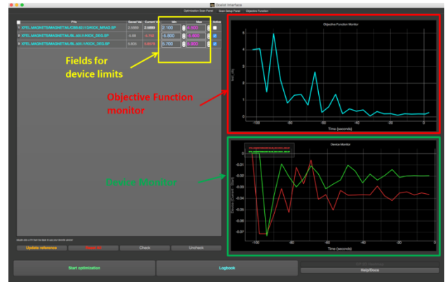
Figure 3: The generic optimizer GUI and dispersion optimization after the laser heater
