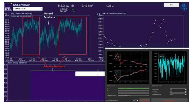
Figure 7: Example of adaptive feedback during European XFEL operation. Lower right corner shows the GUI featuring the current reference and measured orbit, and the photon pulse energy monitor.
