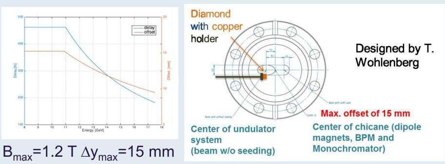
A shift of 7.5 mm is applied to chicane chamber center - > both the dipole magnets and the BPMs are shifted by 7.5 mm to insure a maximum offset of 15 mm
