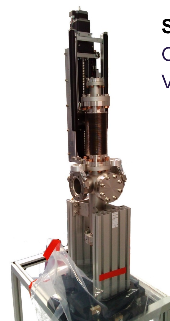
Filter chamber Final vacuum test pending
