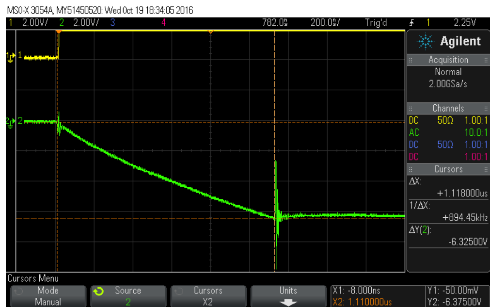
Figure 3.4: Potential measured directly on the electrode of the C1 capacitor, using a 1 MOhm scope-probe ( AC mode). V_{LED\ pulse} = 24\text{ V} , pulse width 1116.83 ns (JDDD=120). The oscilloscope is triggered from an additional output of the ETA-board.
