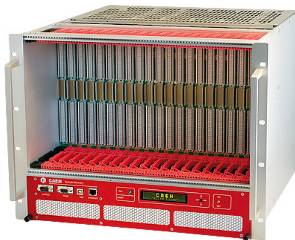
Figure 6.1: Example of a crate (in this case in the VME standard) consisting of a metal frame, a backplane with connectors to connect the inserted modules and a power supply with fan unit (source: http://www.caen.it )
