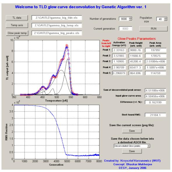
Figure 11: Deconvolution of Gamma – dose 462 mS
