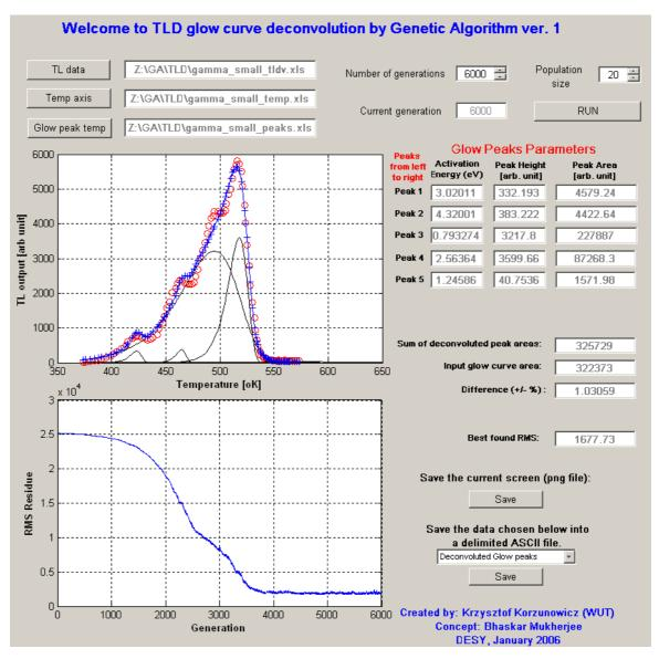
Figure 10: Deconvolution of Gamma data - dose 27.8 mGy
