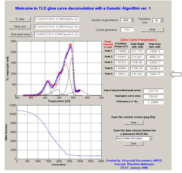
Figure 8: Deconvolution for Polyboron shield (Test 1) – marked neutron Peak
