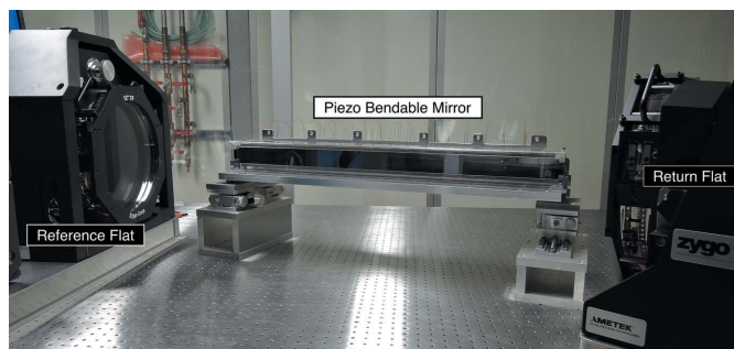
Figure 5 Photograph of the piezo bendable mirror placed in between two auxiliary optical flats, making a cavity in a grazing-incidence setup.
