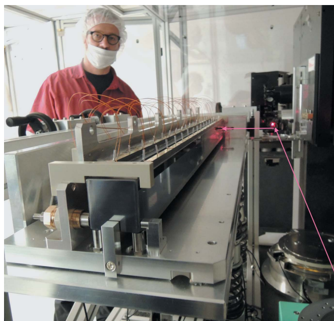
Figure 1 Photograph of the piezo bendable mirror placed in front of the BESSY-NOM. The measuring beam path is sketched in red. The measurement beam is guided in the face side direction by a 45° double-mirror setup, reflected with a normal angle from the mirror surface.
