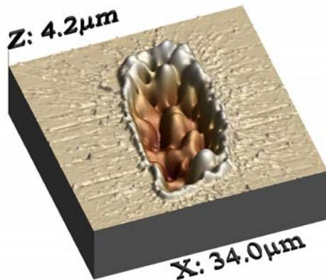
**Figure 2:** PMMA ablated by LCLS tuned at 1.5 nm.
