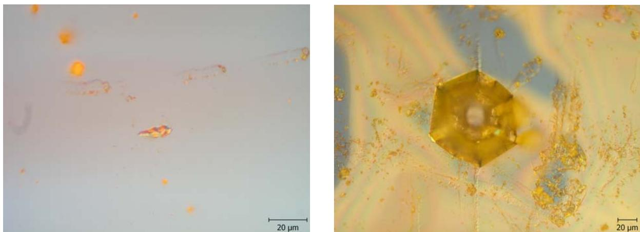
**Figure 5:** DIC images of PbI<sub>2</sub> irradiated (left) near and (right) above the damage threshold by 800-eV LCLS radiation.
