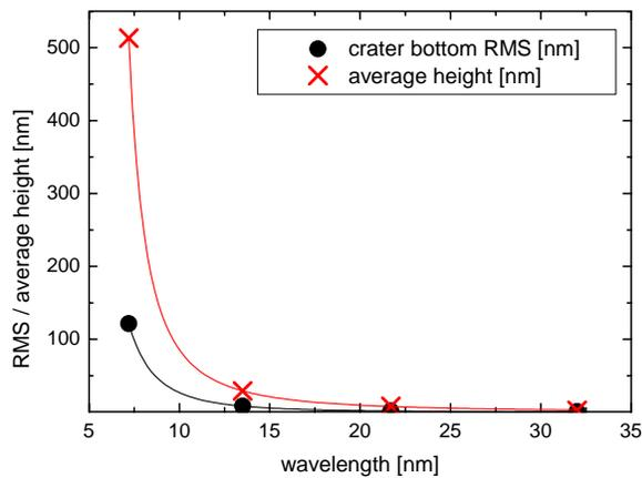
**Figure 1:** Wavelength dependence of a roughness of PMMA ablated at FLASH tuned from 32 nm to 7.1 nm.
