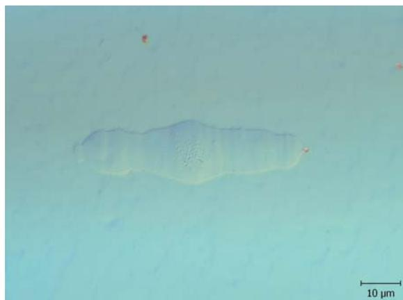
**Figure 3:** The DIC image of a crater formed in  $\text{PbWO}_4$  by the focused LCLS beam near the ablation threshold.
