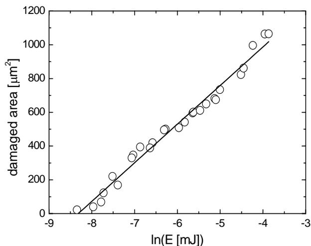
**Figure 4:** The dependence of  $\text{PbWO}_4$  surface area damaged by 800-eV LCLS radiation on the pulse energy.
