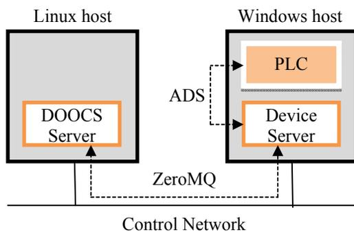
Figure 1: Integration of undulator control into DOOCS.
