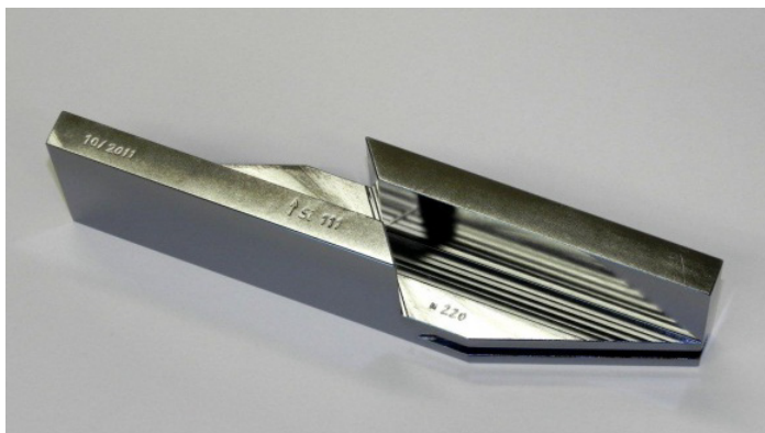
Figure 10: Si(111) channel-cut crystal
