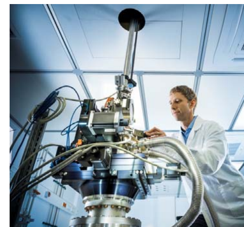
Compact pulsed magnet for MID and SCS: 15 Tesla 0.6 ms pulse length sample at 4.2 – 300 Kelvin
