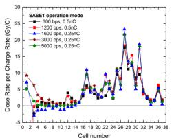
Figure 2: SASE1 dose rate per charge rate during selected operating modes at different repetition rates. Cell#1 corresponds to the DU location.
