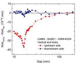
Figure 4: Measurable magnetic field integral changes are seen in Cell#3-SASE1 segment after exposed to about 230 Gv.
